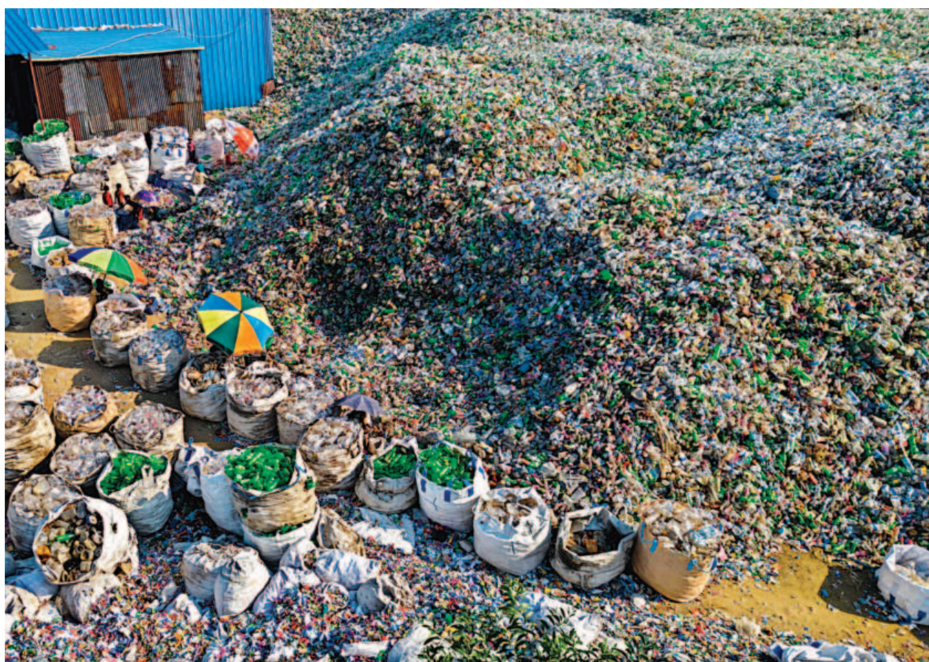
Discarded plastic bottles are brought to a recycling factory in Chattogram city's Bakalia area, where they are cut into small pieces, washed, and dried into flakes before being packed and exported abroad. This recycling process helps reduce pollution and has also created employment for people.
