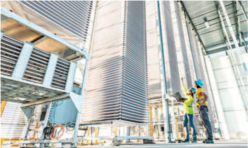
A person points at a stack of trays holding treated limestone, used to absorb CO2 from the air, at a plant in Tracy, California.
