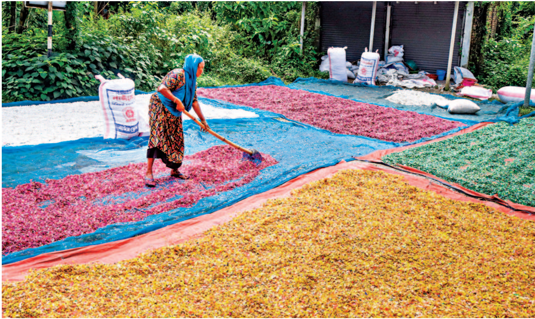
A worker spreads out shredded plastic under the sun to dry. Discarded plastic is sorted based on the chemical properties and colour, shredded into pieces, washed and then placed into machines which melt and inject them into moulds, creating everyday items used around the house. Each kilogramme of such shredded plastic sells for anywhere for Tk 35 to Tk 110. The photo was taken at Aronghata Lata Mor in Khulna recently.
