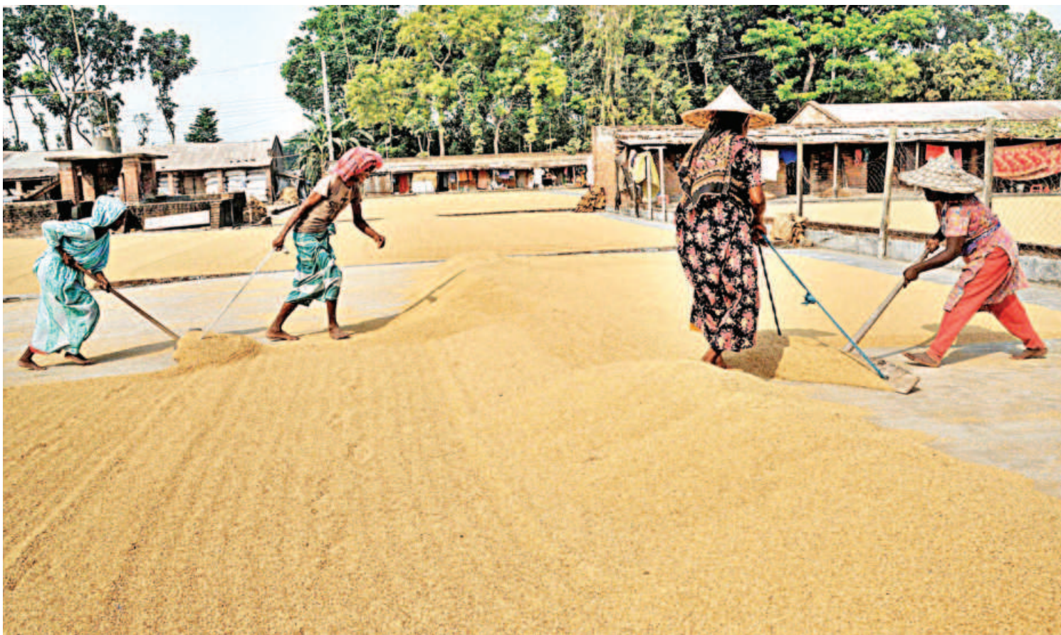
Workers spread paddy out in a courtyard of a rice mill to dry under the sun in Naohata area of Rajshahi's Poba upazila. The milling process involves cleaning of paddy, soaking, steaming, draining of water, sun drying, milling, aerating and bagging. With the advent of machines, scenes like these are turning less common. The photo was taken yesterday.
