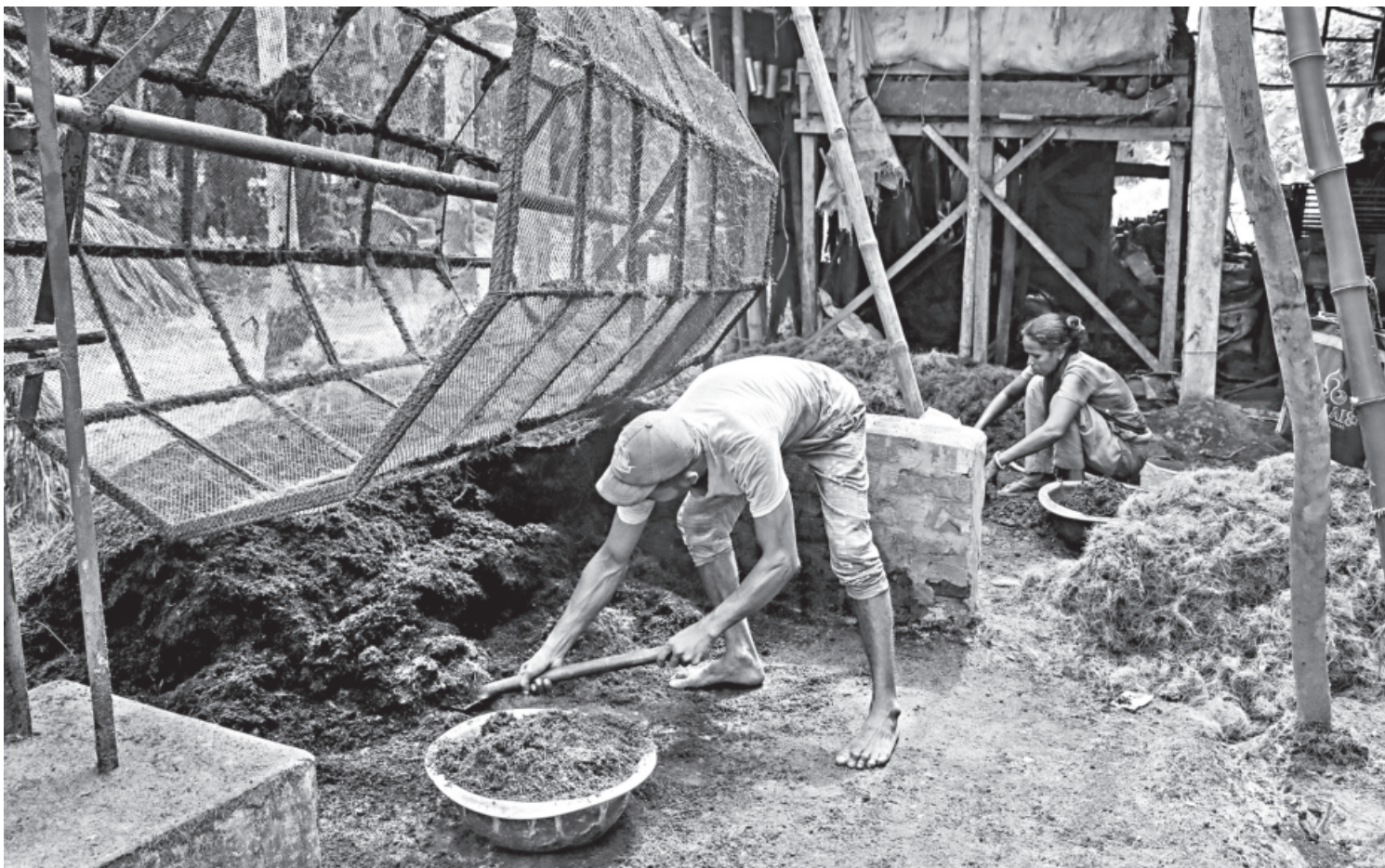
Labourers in the process to produce cocopeat from coconut coir at Rahimabad village in Bagerhat, Khulna, yesterday. Local entrepreneurs collect, dry, and refine coconut husks to make cocopeat, a popular soil substitute in agriculture, nurseries, and rooftop gardens for its excellent water-retention properties.
