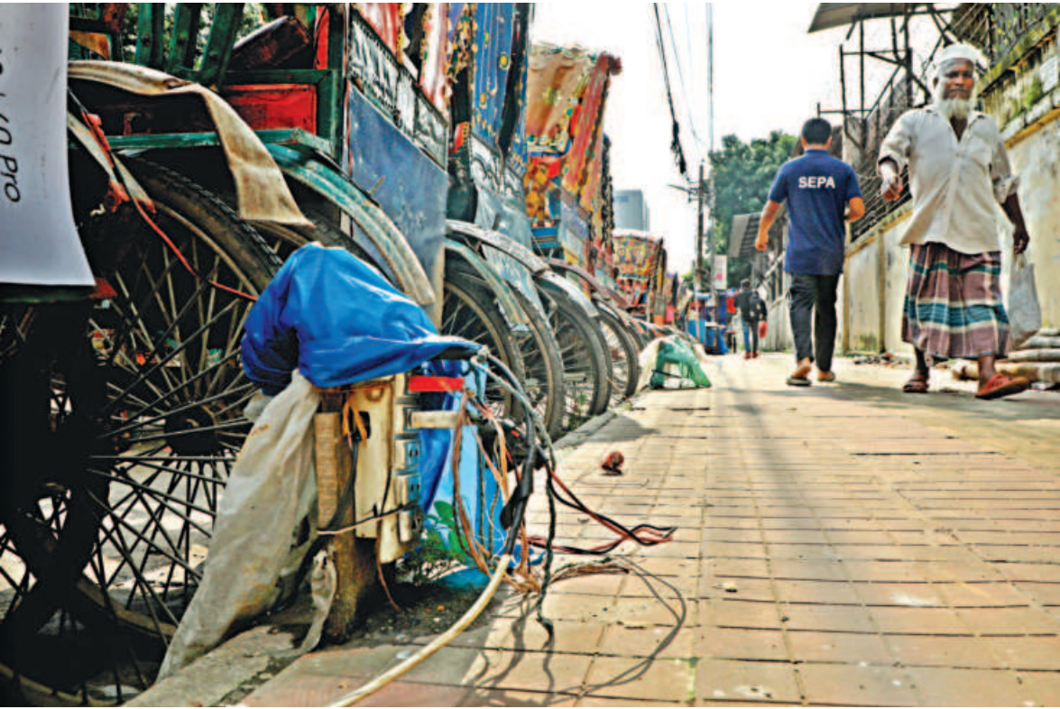
This makeshift charging rig for battery-run autorickshaws on a pavement poses a risk of electrical short circuits and electrocution, potentially leading to accidents involving pedestrians. The photo was taken recently in the capital's Tejgaon Industrial Area.
