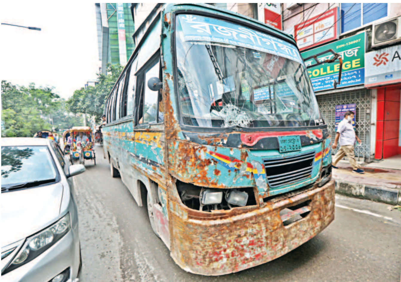
Despite broken headlights, a cracked windshield, and rust covering its body, this bus continues to operate in the capital. Public transport vehicles are required to pass a mandatory fitness test, and since July 21 the government has announced strict penalties for operating ramshackle buses and trucks with faulty machinery. Yet such dilapidated buses still ply the city's streets. This photo was taken in Lalmatia yesterday.
