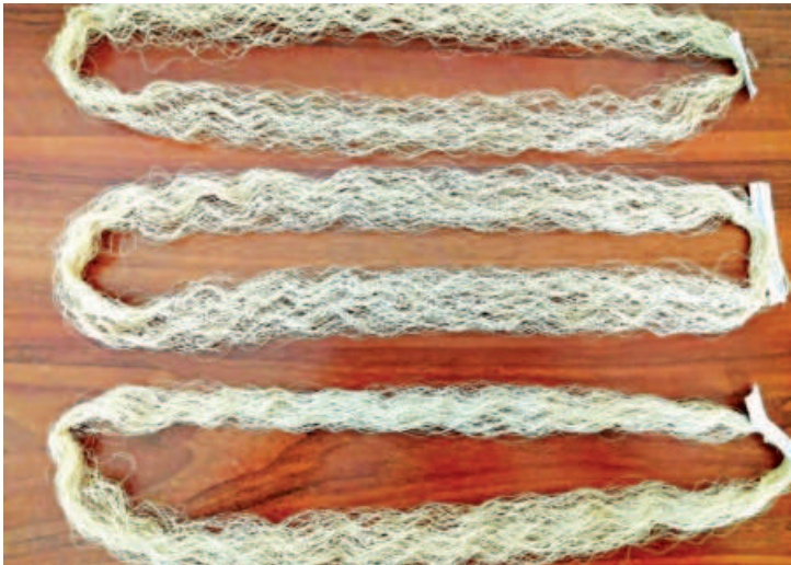
Threads are gently hand-rolled, dried, and spun into thread using spinning wheels.
