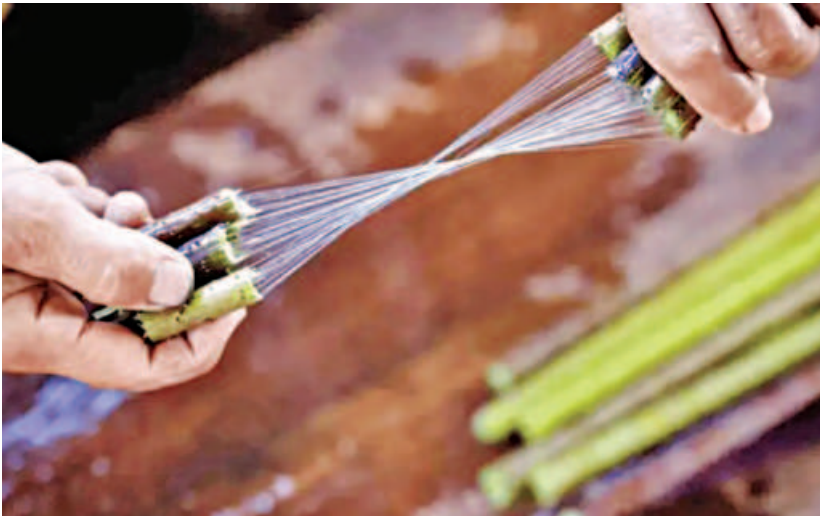
Inside the stem are sticky threads that, once exposed to air, turn into fine filaments.
