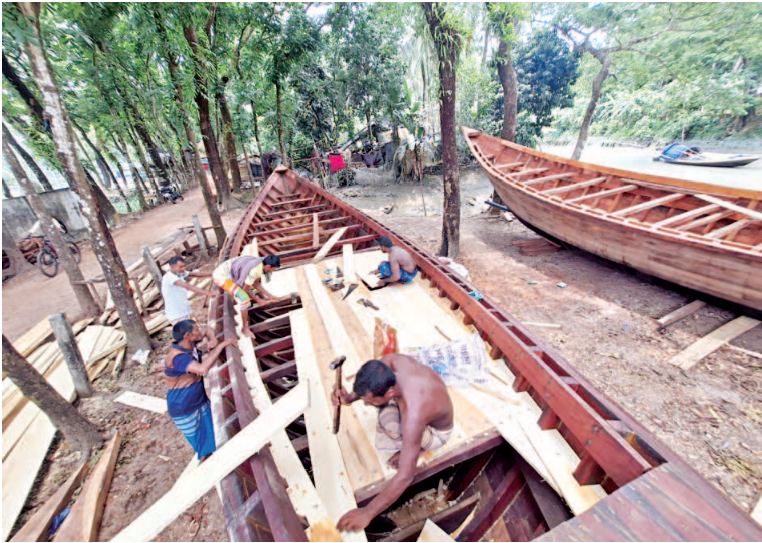
Workers earn Tk 1,000 a day to build 15-by-45-foot fishing boats using mahogany and chamble wood. Each boat, made over 15 to 20 days, is sold to fishermen for Tk 1.6 lakh. The photo was taken in Chandramohan area of Barishal sadar upazila recently.
