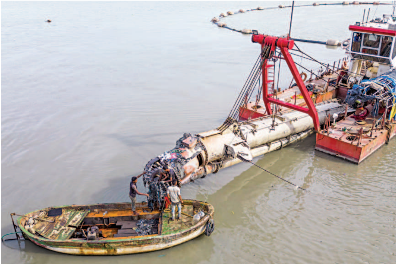
The ongoing capital dredging of the Karnaphuli is being repeatedly hampered by polythene and waste clogging the machine, forcing frequent shutdowns and slowing progress. On International Day for Biological Diversity today, the river's condition stands as a stark reminder of how pollution endangers both development and biodiversity. The photo was taken yesterday afternoon.
