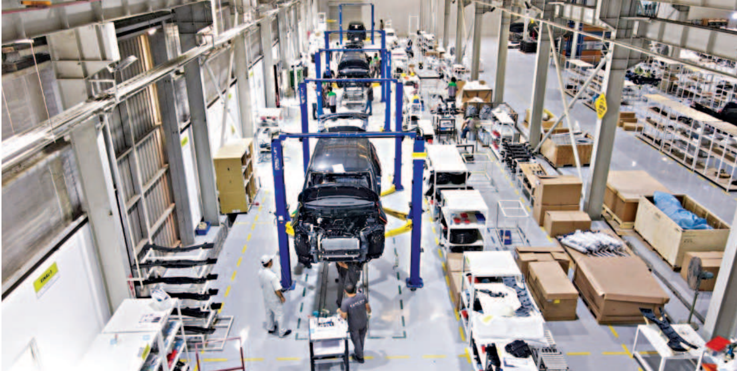
Employees and machines work in harmony at an assembly line at the Rancon Auto Industries facility, located within its industrial park in the Kashimpur Union of Gazipur. In addition to assembly and inspection, the factory is now capable of painting certain models, including those of brands such as Mitsubishi and Proton.
