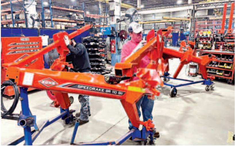
Workers install parts on a hay rake, used by farmers to collect hay or straw into rows for easier baling, inside Kuhn North America’s factory in Brodhead, Wisconsin on March 6.
