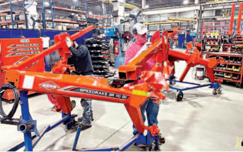
Workers install parts on a hay rake, used by farmers to collect hay or straw into rows for easier baling, inside Kuhn North America’s factory in Brodhead, Wisconsin on March 6.
