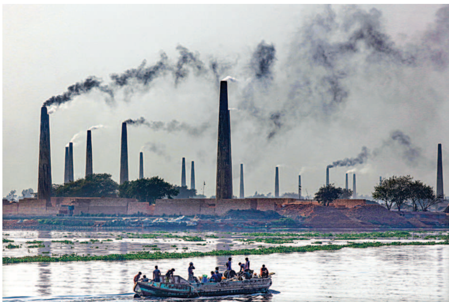
The sky is overcast by the plumes of smoke from the brick kilns in the Fatulla area of Narayanganj. Most of these kilns burn wood, coal and other fossil fuel using traditional method, which creates more smoke and deteriorates the air quality. The photo was taken last week.
