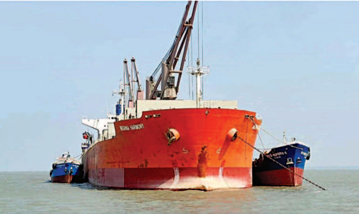
Goods are unloaded to lighter vessels at the outer anchorage of Payra port in Patuakhali as reduced navigability bars ships with a 10.5m draft from reaching the main jetty. Photo was taken recently.
