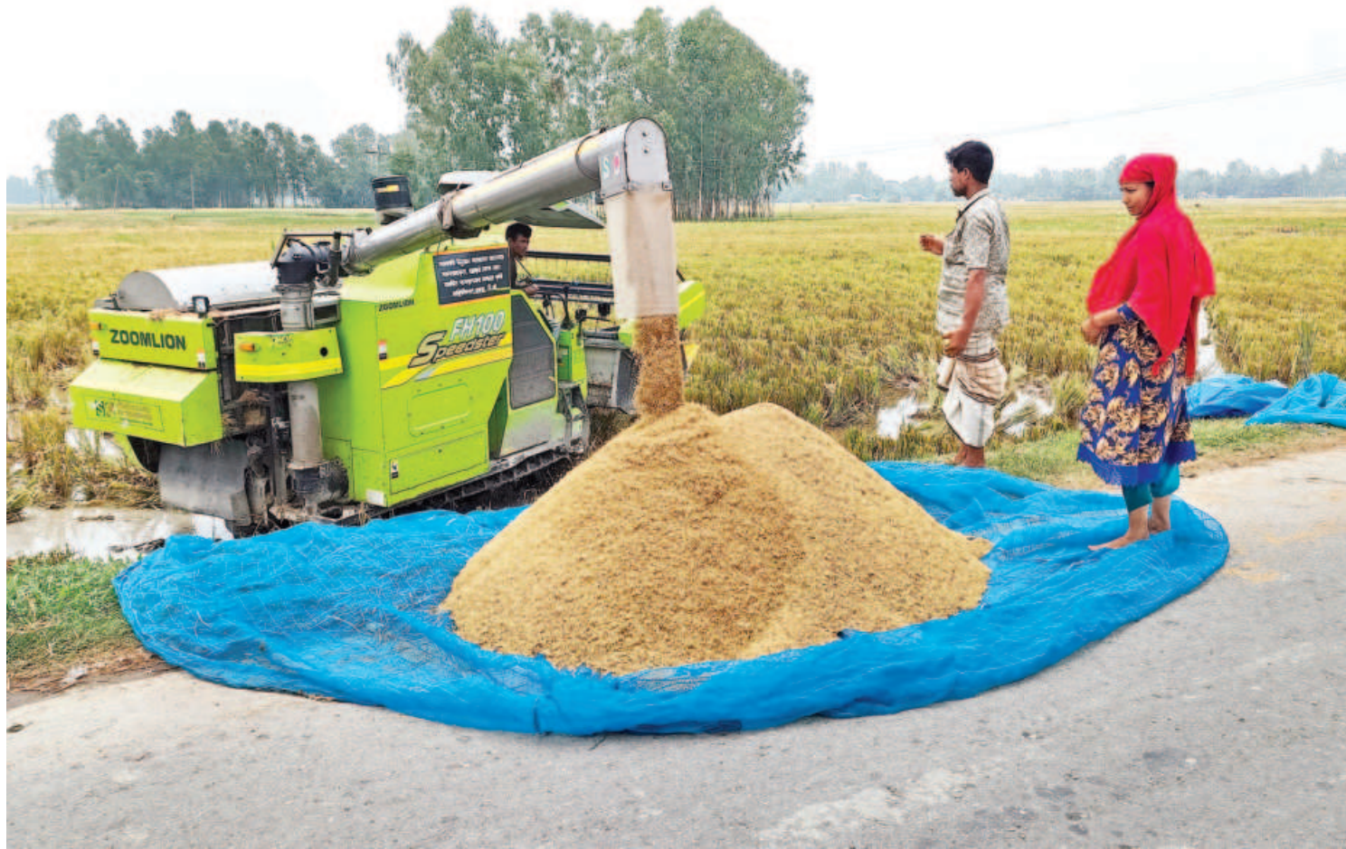
Farmers gather paddy using a combine harvester at Gobindaganj upazila of Gaibandha. The farm machine both cuts the paddy and threshes grain, helping to save on time and cost of labour. The photo was taken a couple of months ago.
