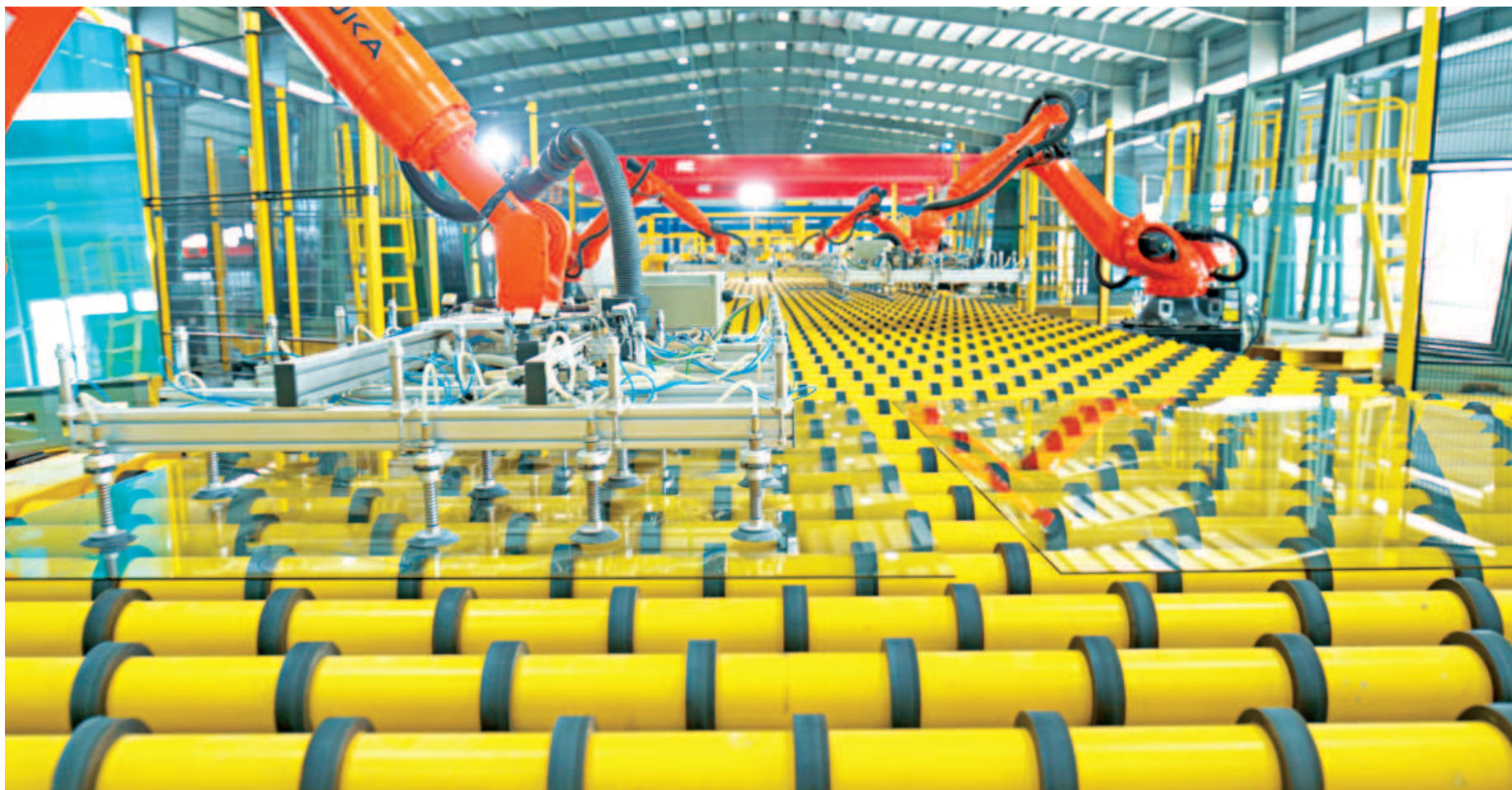
The interior of AkijBashir Group's glass-manufacturing factory, located in Habiganj's Madhabpur, features impressive technologies to enhance product quality, including an online scanner that checks panes for impurities like bubbles or stones. PHOTO: COLLECTED
