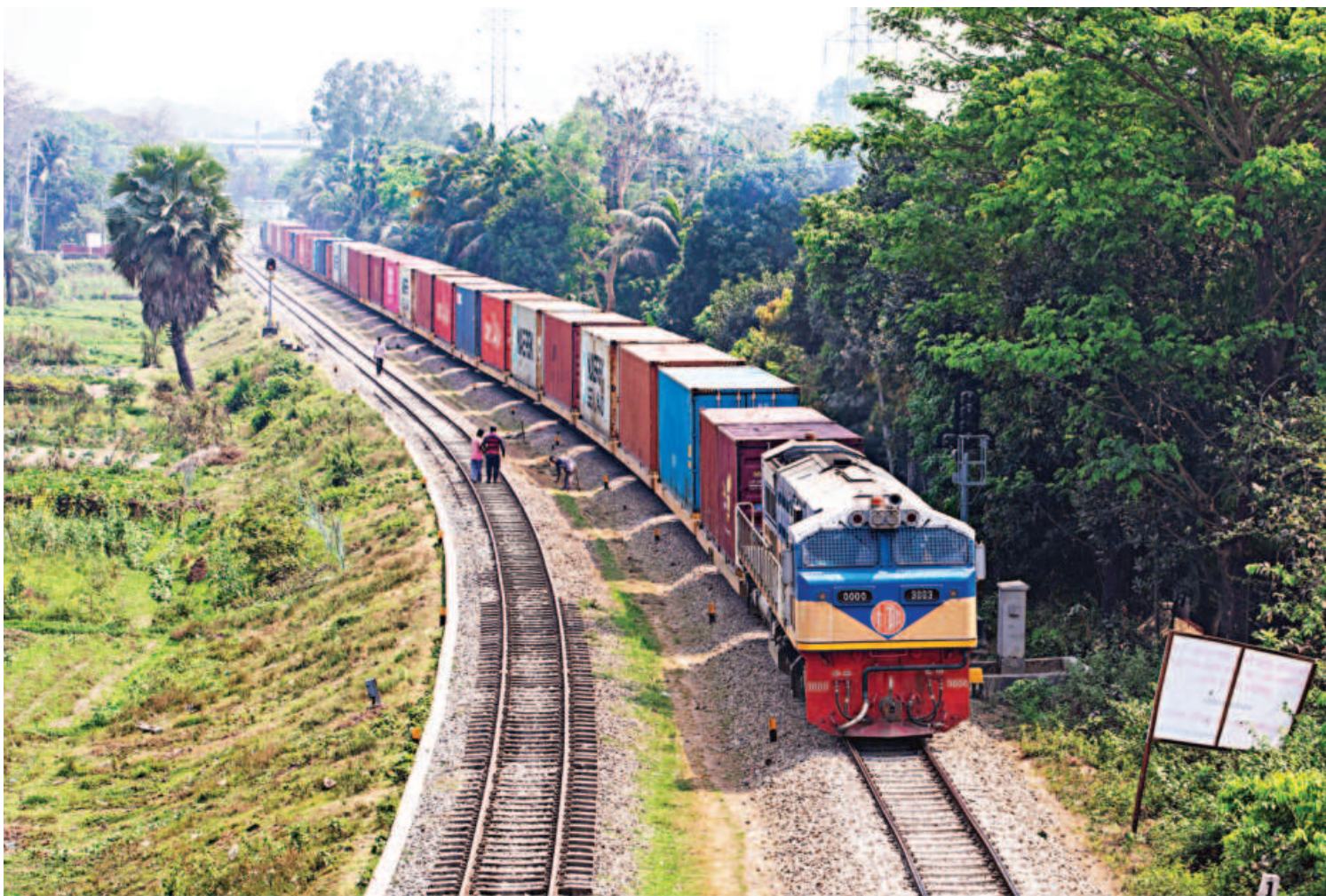
A locomotive engine pulls 31 wagons, each of which can accommodate a 40-foot equivalent unit of container. This means that more than 31 containers can be transported when dealing with 20-foot equivalent units, excluding those carrying heavy loads such as machineries and steel coils. Nowadays, around three to four freight trains are departing the Chattogram port for Kamalapur in Dhaka each day. PHOTO: STAR/FILE
