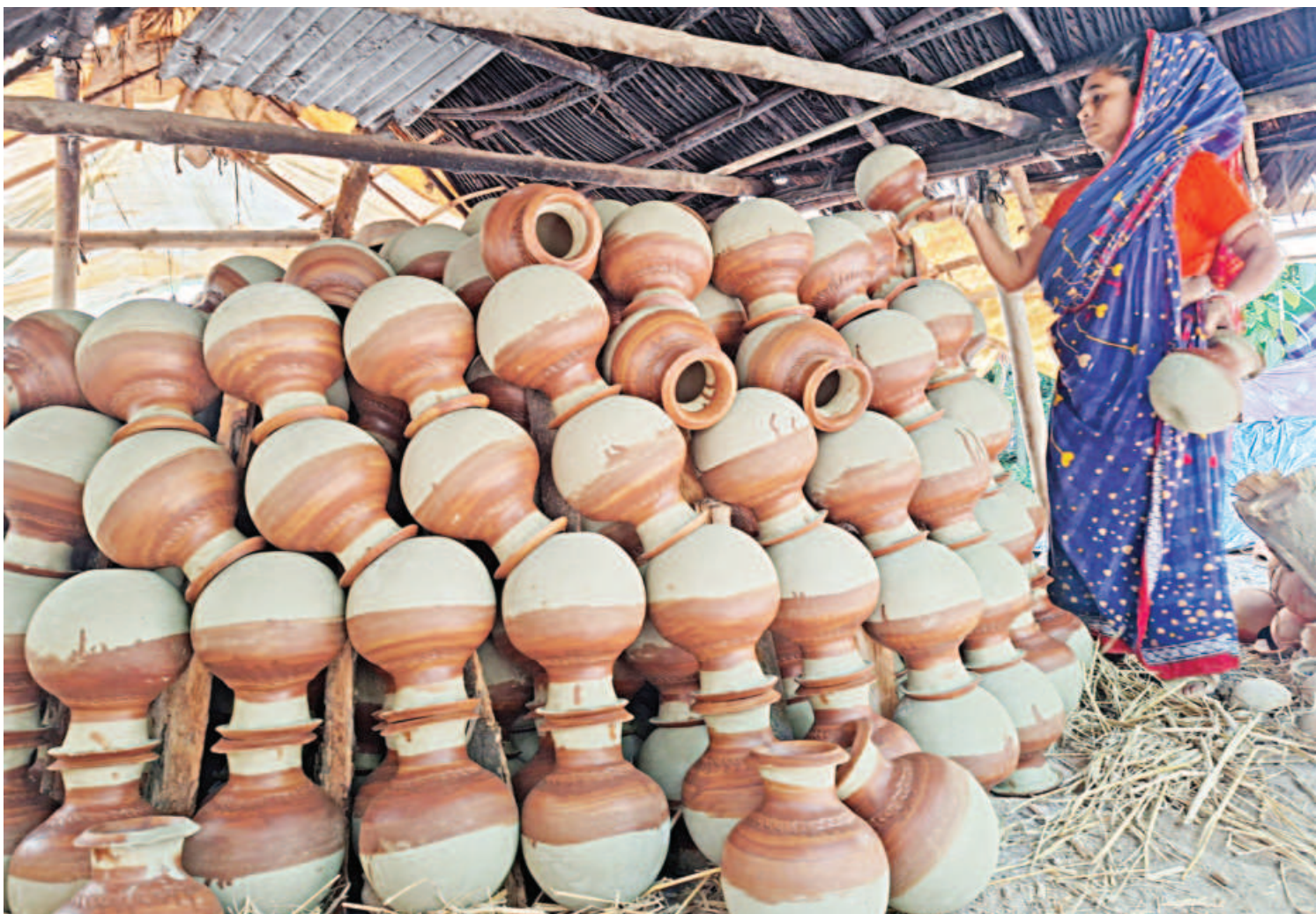
Potter Laxmi Rani stacks clay pitchers in order to bake them in an open fire, an arrangement locally known as "puin". Each pitcher sells for Tk 15 to Tk 20 at wholesale. The photo was taken at Shimuleshwar village in Jhalakathi district recently.
