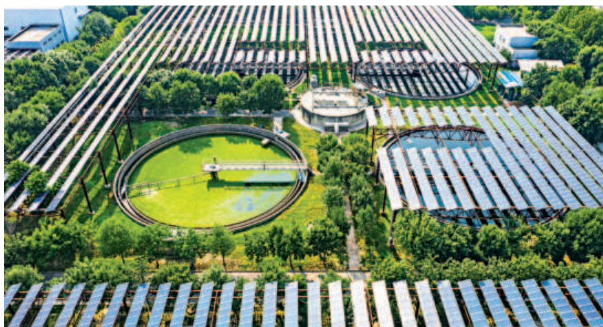
This aerial photo shows solar panels built over a sewage treatment plant in Zhengzhou, China's central Henan province. China is building almost twice as much wind and solar capacity as every other country combined.
