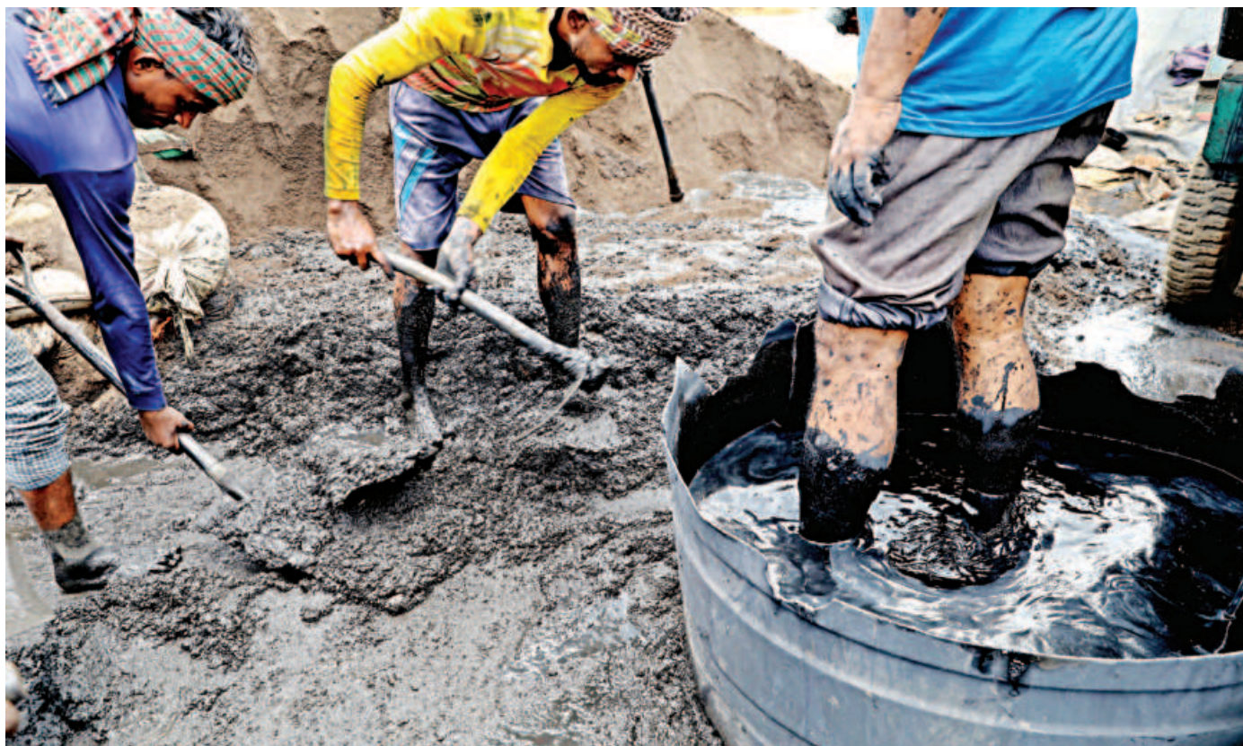
At a makeshift recycling shop, workers separate scrap metal and a cement-like substance from waste generated by steel re-rolling mills. While the recycled materials find their way back to steel mills and construction industries, the recycling process itself raises serious health concerns. The photo was taken in Kutubpur area in the capital's Shyampur yesterday. PHOTO: ANISUR RAHMAN
