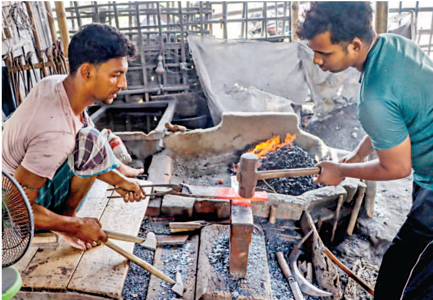
Blacksmiths are busy hammering a hot piece of metal into a traditional meat cleaver, one of the largest kitchen knives with a broad blade meant for cutting animal carcasses into pieces. Sold by weight, such cutting tools can cost anywhere from Tk 500 to Tk 800 per kilogramme. The shop hopes to make sales of around Tk 30,000 to Tk 40,000 centring the sacrifice of cattle marking Eid-ul-Azha next week. The photo was taken from Khulna's Dumuria upazila recently.
