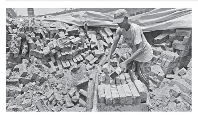
These bricks were shaped and left to dry before placing them in the furnace. However, in the aftermath of Cyclone Remal, most of the bricks turned into clay due to excess rain. Now, workers are extracting the ones that have preserved their shape. The photo was taken the Doarika area of Barishal yesterday.
