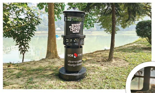
light at a particular wavelength which enables it to interact with a special chemical coating within the device. Scientifically, this interaction is called photocatalysis.
