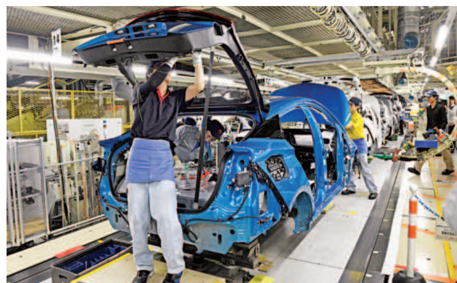
Workers assemble fourth generation Toyota Prius cars on the production line at the company's Tsutsumi assembly plant in Toyota City.
