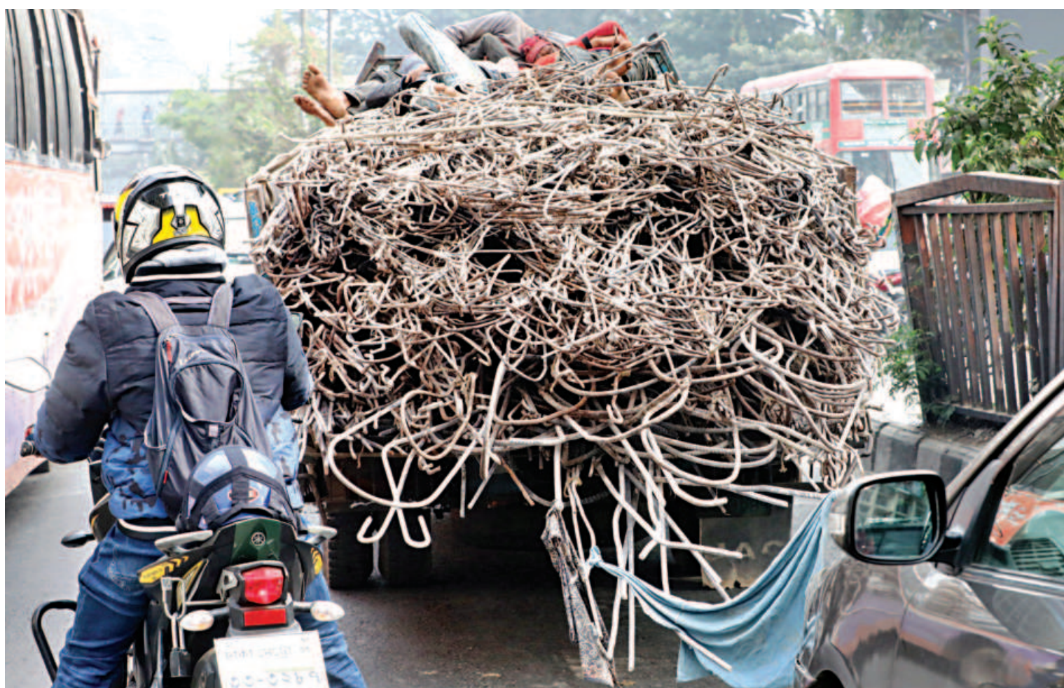
Steel rods being openly carried on a truck with a car trailing right behind in the capital's Shahbagh. One strong jerk, and the rods could easily slide off and pierce right through the vehicle at the back. Timber and rods are often carried with no precautions in place, increasing the risks of accidents.
