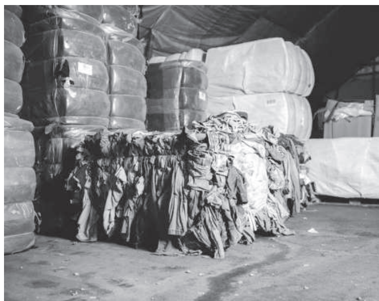
Renewcell developed a process to recycle cotton-rich clothing to produce Circulose, a dissolving pulp that can be used to make man-made cellulosic fibres.
