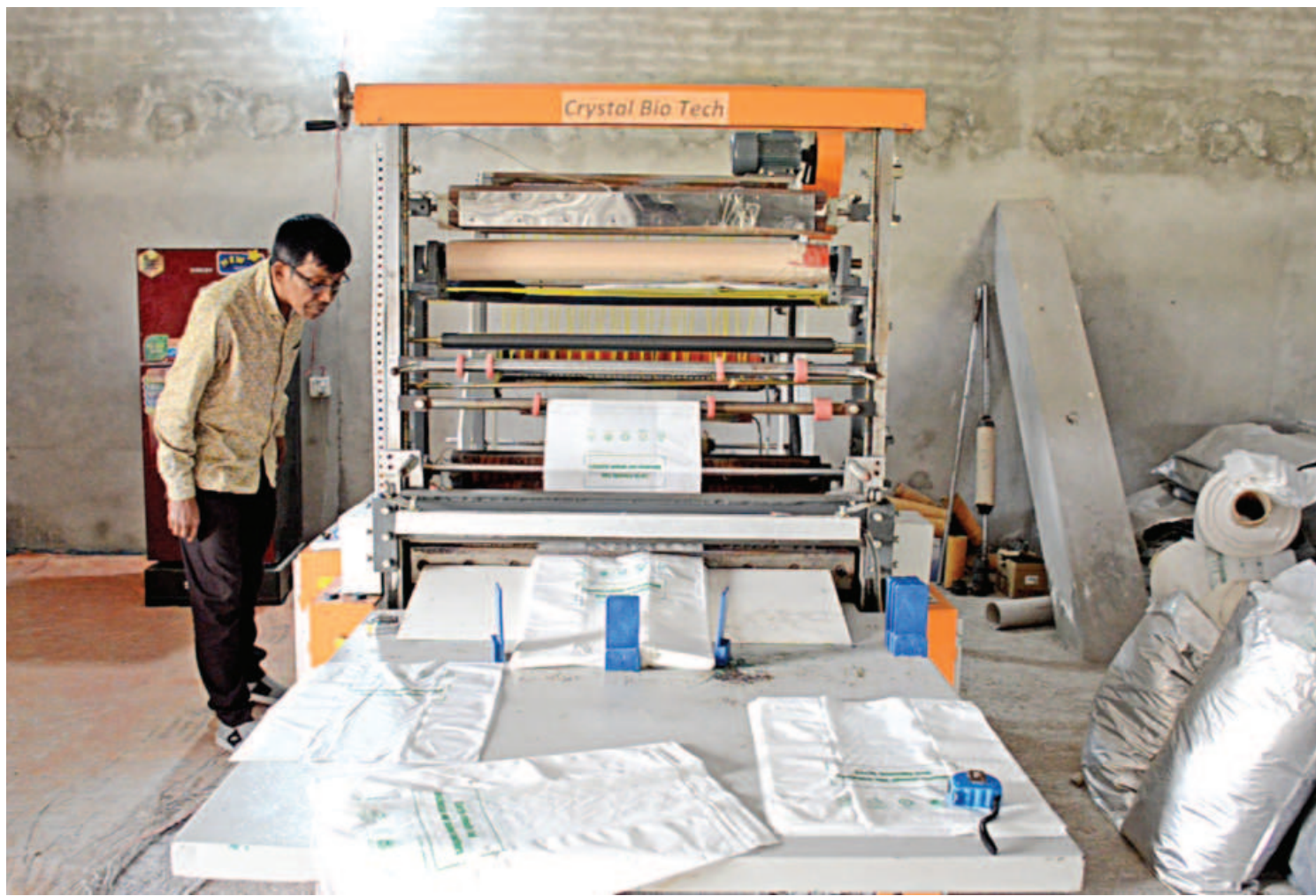
A worker inspects compostable bioplastic bags made from corn starch granules at the Crystal Bio Tech factory in Godagari upazila of Rajshahi. Despite being an alternative to polyethene products, the factory has been unable to enter commercial production in absence of "green" certification.
