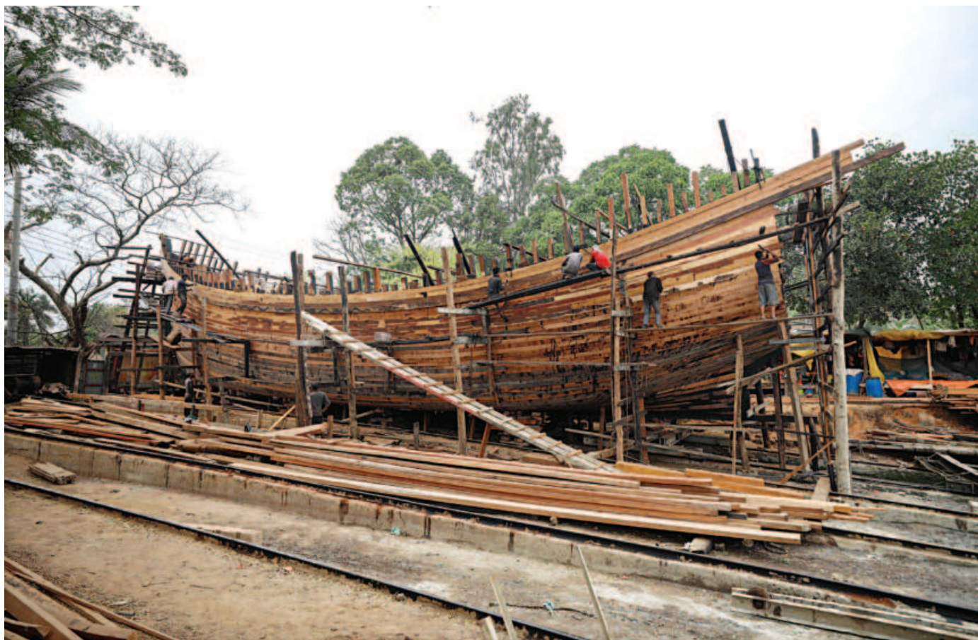
Craftsmen are making a wooden boat which will be used to bring brine from the islands to the refineries in Chattogram. Owners say 95 feet long and 35 feet tall boat costs over Tk 2 crore to make at the dock in Kalurghat area of the port city. The photo was taken last week.
