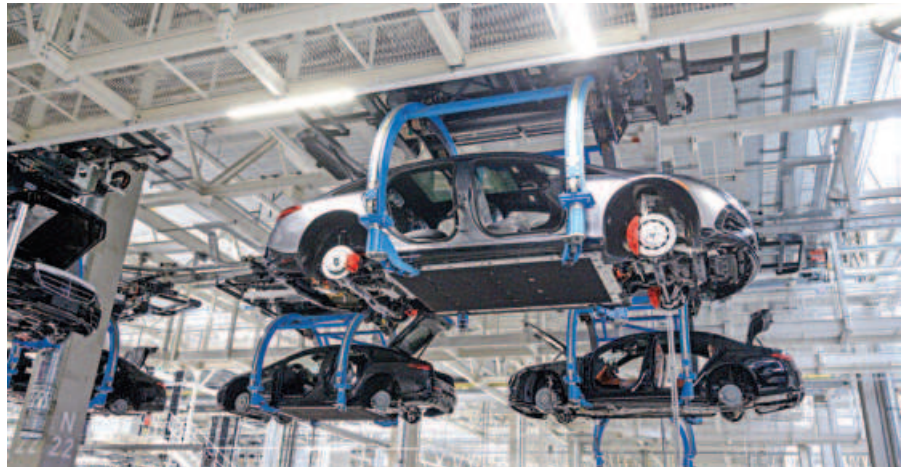
Mercedes-Benz EQS and S-Class passenger cars are transported automatically to their next production step at a digitised assembly line, in Sindelfingen, southwestern Germany.
