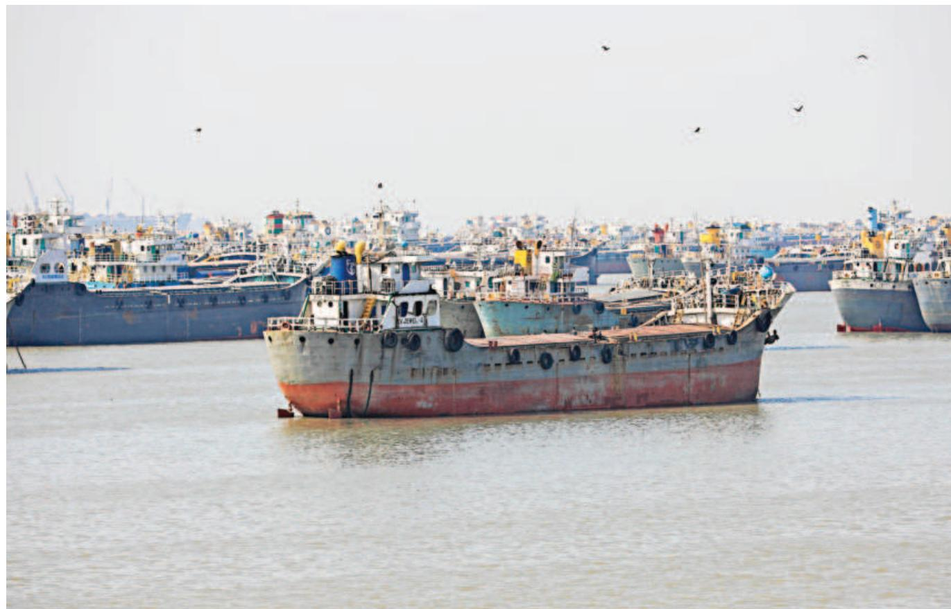
**Lighter vessels are used to unload a major portion of imported goods, including industrial raw materials, foodgrain and fertiliser, from mother vessels which have to lessen their load at the outer anchorage to meet the draught limit for entering the Chattogram port. Having carrying capacities of 1,000 to 2,000 tonnes, these lighter vessels then transport the goods to different destinations around the country over inland waterways. The photo was taken at Patenga last week.**
