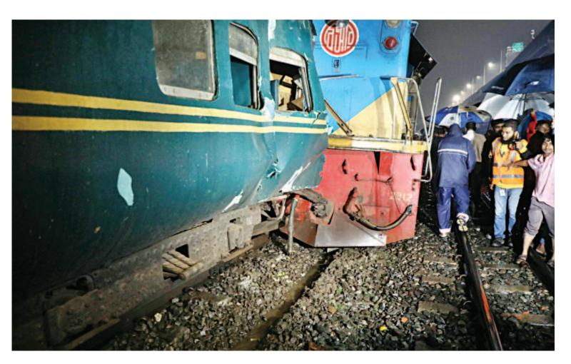
The locomotive and a carriage of Titas Commuter train derailed under the Dhaka Elevated Expressway near Tejgaon Railway Station yesterday evening after the train hit a crane being used in the construction of the expressway as the latter was crossing the rail track. The accident snapped rail communication between Dhaka and the rest of the country for five hours from 5:00pm. PHOTO: PRABIR DAS
