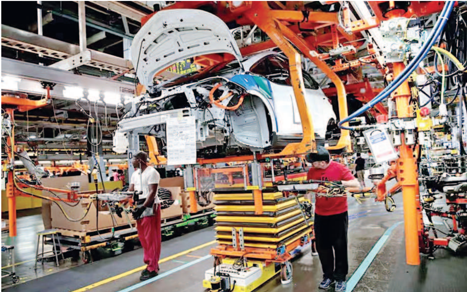
General Motors assembly workers connect a battery pack underneath a partially assembled 2018 Chevrolet Bolt EV on the assembly line at Orion Assembly in Lake Orion, Michigan, US on March 19, 2018. US Treasury will temporarily exempt some trace critical minerals under strict new rules barring materials from China and other countries.
