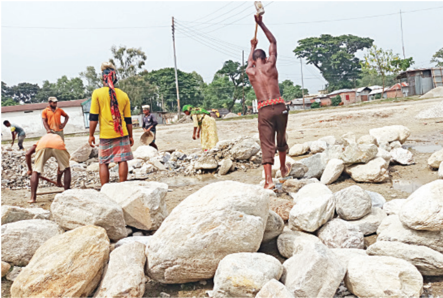
Stone crushers at Burimari land port in Patgram upazila of Lalmonirhat are seen breaking boulders into bits that can be run through grinding machines to produce smaller sized stones used in construction. Although the backbreaking work entails heavy labour, these workers are denied proper pay in absence of other lines of work in the region.
