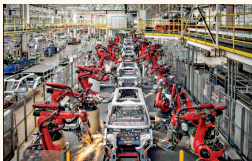
Robotic arms assemble cars in the production line for Leapmotor's electric vehicles at a factory in Jinhua, the Zhejiang province of China.
