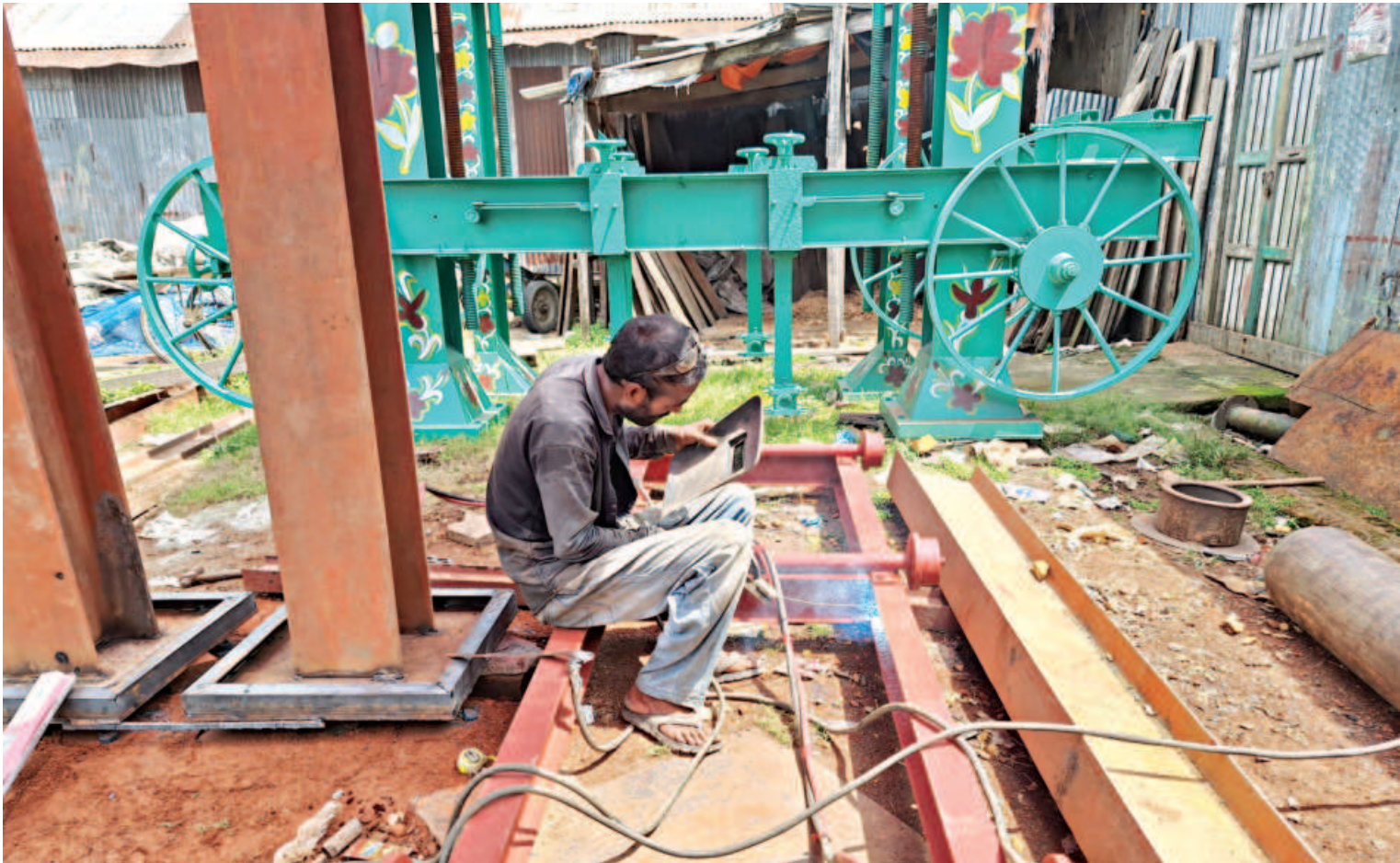
Nantu Sarder fabricates a trolley for a band saw machine, which is principally used in woodworking, metalworking, and lumbering, but may cut a variety of materials. A craftsperson can create the whole setup in around 40 days, receiving around Tk 31,000 for the effort from the shop owner. The photo was taken next to Banaripara upazila launch terminal in Barishal last week.
