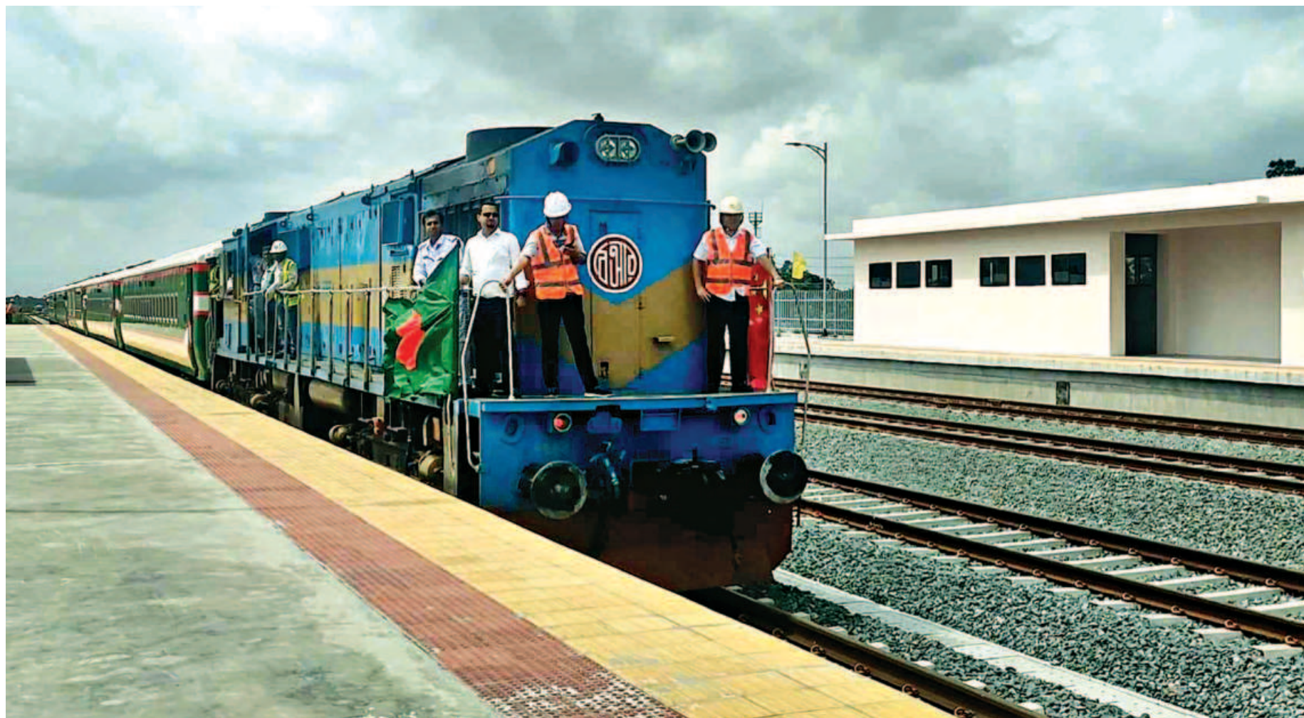
A Bangladesh Railway train testing the speed limit on the newly constructed Mawa-Bhanga rail line yesterday. The train went back and forth between Mawa Railway Station in Munshiganj and Bhanga Railway Station in Faridpur through the Padma Bridge at different speeds.
