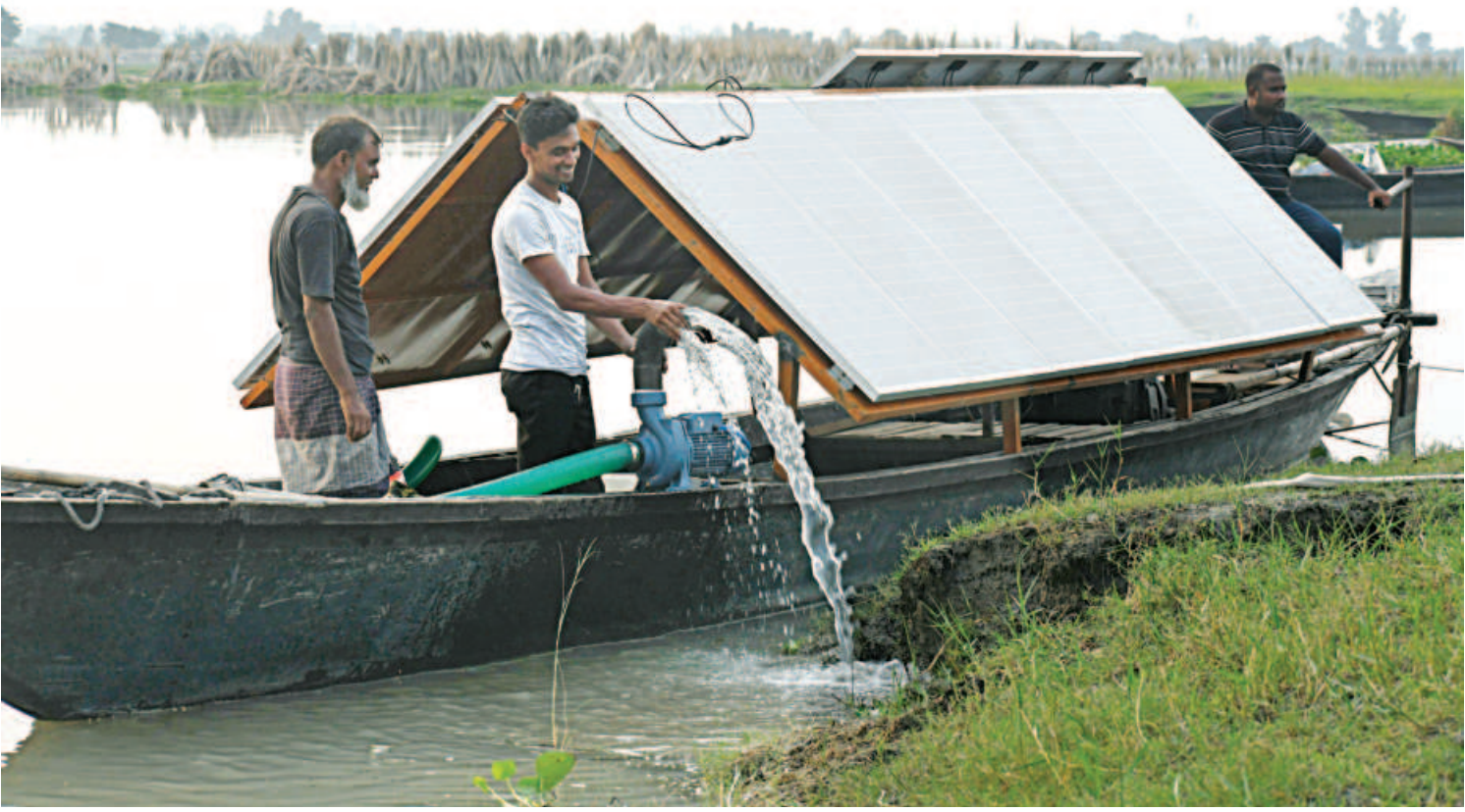
A solar-powered pump set up on a boat to act as a mobile irrigation facility for croplands in chars. The 5-kilowatt pump can irrigate 40-50 bighas of land and costs Tk 2.5 lakh to set up. The facility came about under a one-year research project being jointly implemented by Rural Development Academy Bogura, Chars Development Research Centre and United Commercial Bank. The photo was taken at Noapara Char of Bogura's Shariakandi upazila on Wednesday.
