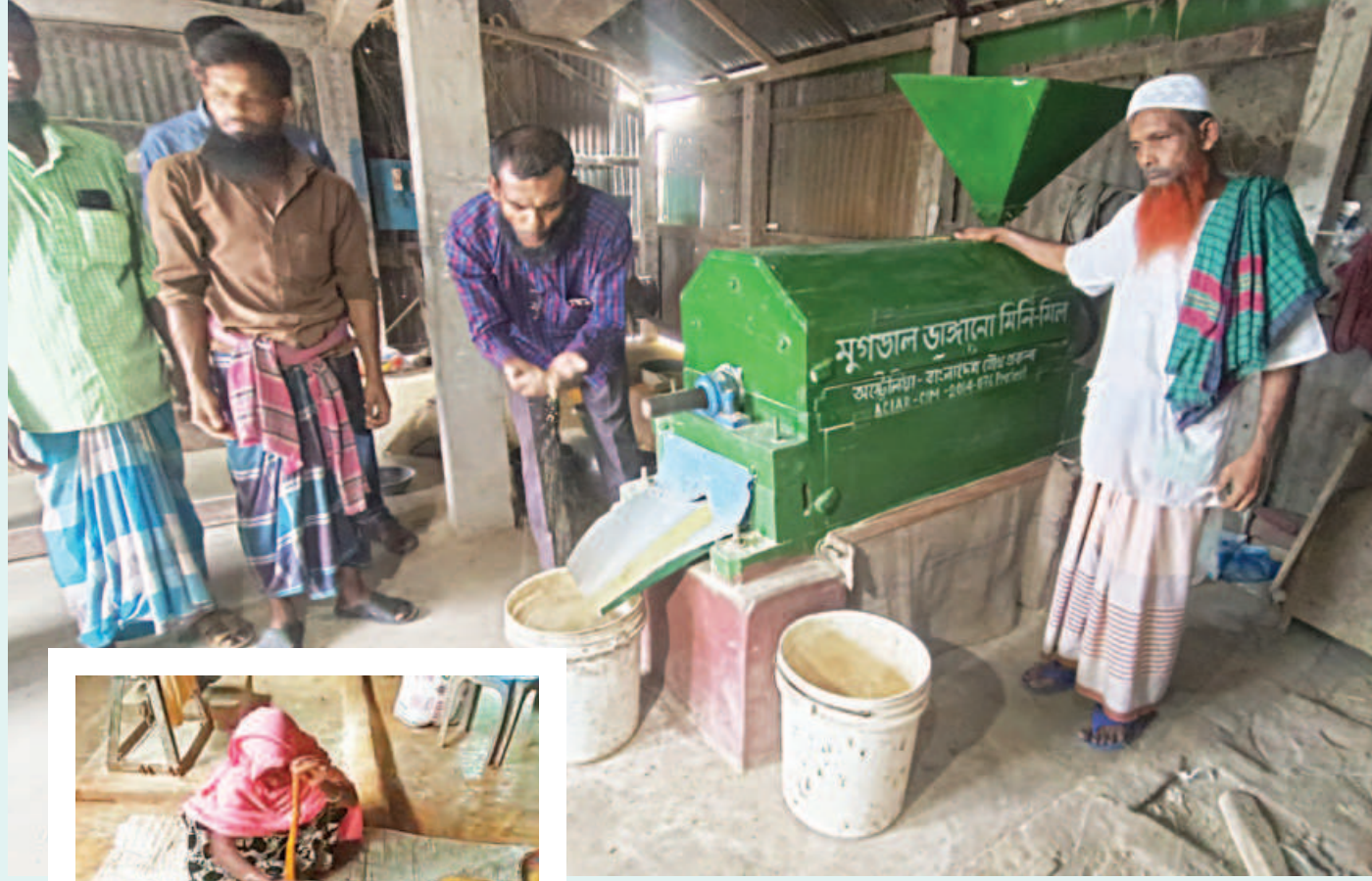
Mung dal being processed from mung bean using a milling machine developed through a project undertaken by the Bangladesh and Australian governments. Inset, until a couple of years back, quern-stones were used for the purpose. PHOTO: SOHRAB HOSSAIN
