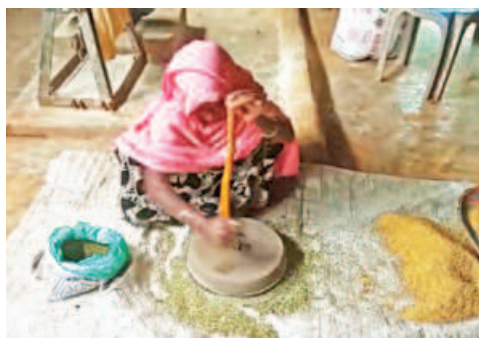
Mung dal being processed from mung bean using a milling machine developed through a project undertaken by the Bangladesh and Australian governments. Inset, until a couple of years back, quern-stones were used for the purpose. PHOTO: SOHRAB HOSSAIN
