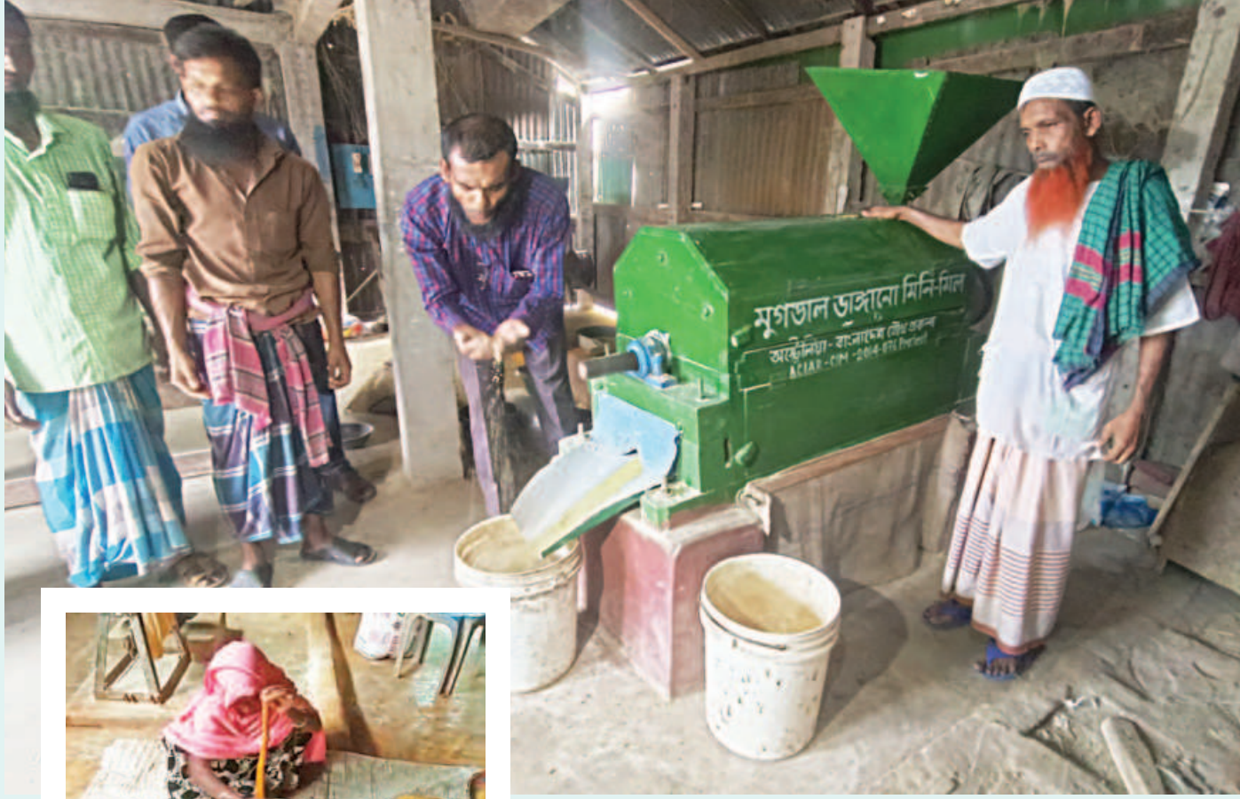
Mung dal being processed from mung bean using a milling machine developed through a project undertaken by the Bangladesh and Australian governments. Inset, until a couple of years back, quern-stones were used for the purpose. PHOTO: SOHRAB HOSSAIN
