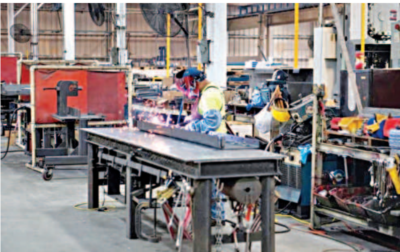
An employee welds a screed bottom for a commercial class road paver at the Calder Brothers factory in Taylors, South Carolina.
