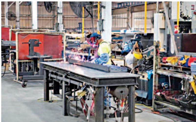
An employee welds a screed bottom for a commercial class road paver at the Calder Brothers factory in Taylors, South Carolina. PHOTO: REUTERS/FILE
