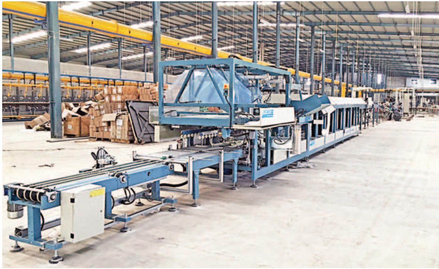
Auto packaging machines are seen at a ceramic factory in Nilphamari. An inadequate supply of natural gas in northern region of Bangladesh is prompting local ceramic makers to come up with alternative sources of fuel that are driving up production costs.
