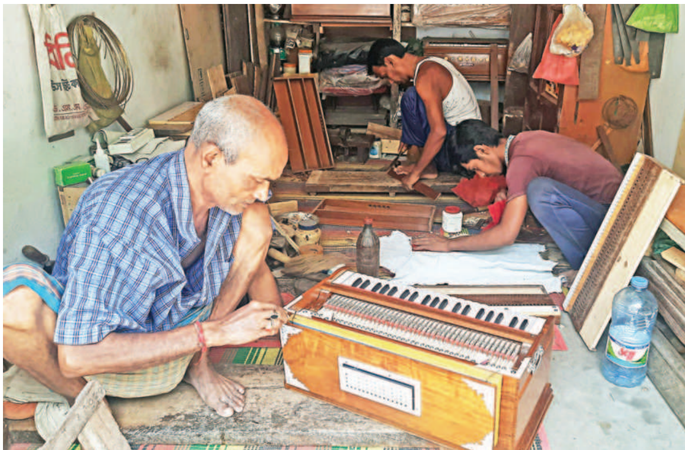
Nikhil Sarker polishes an Indian version of the harmonium, a free-reed aerophone used in music of all kinds, including folk, light, semiclassical and classical. One can take around one month to make out of wood, metal, brass and cloth. The veteran artisan charges anywhere from Tk 25,000 to Tk 60,000 for each depending on the quality. The photo was taken next to Khulna Press Club on Sir Iqbal Road in Khulna city recently.
