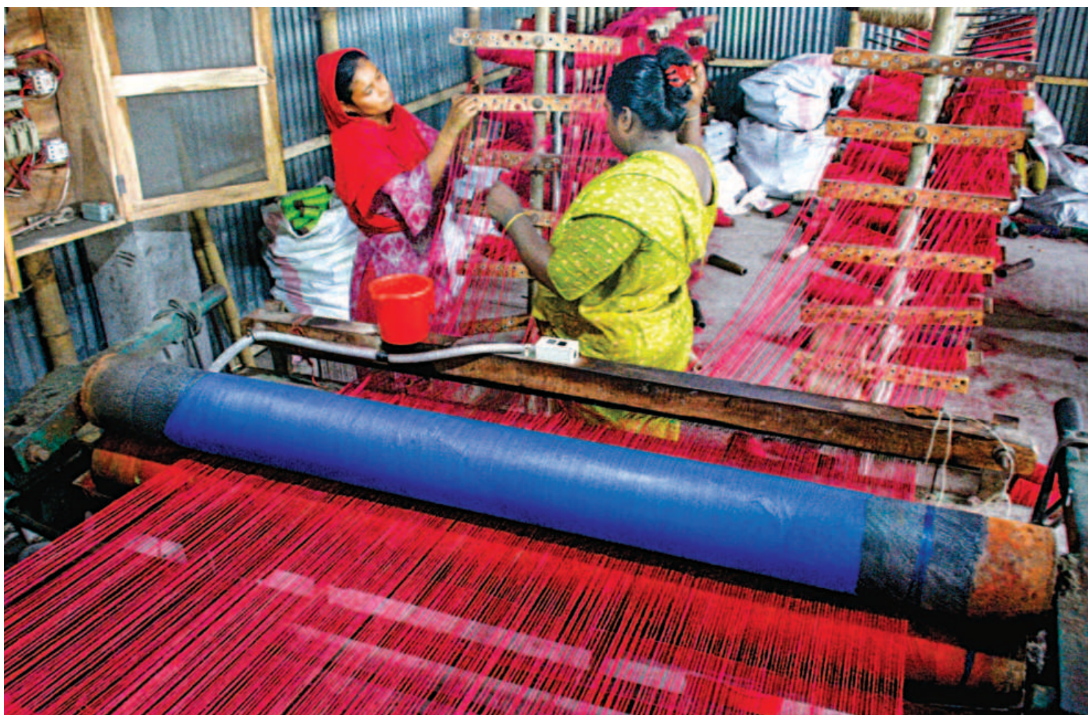
Two women working at a carpet-making factory in Khulna's Boyra Rayermohol area. Bright carpets are being produced after mixing different types of colours with jute yarn. After the closure of jute mills in Khulna, some employees have switched to carpet-making. A machine can manufacture 130 yards of carpet daily and the wholesale price of each yard is Tk 110. The photo was taken recently.
