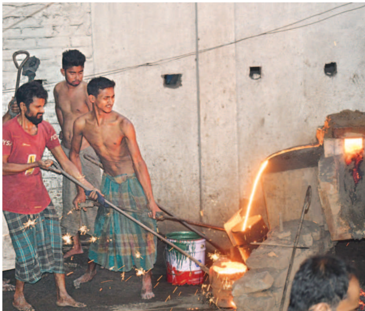
Workers are seen melting iron before reshaping it for use in building agricultural machinery. Many foundries in Bogura have been fitted with latest induction furnaces and computerised numerical control machines to ensure that the quality of their products can rival that of any imported alternatives.
