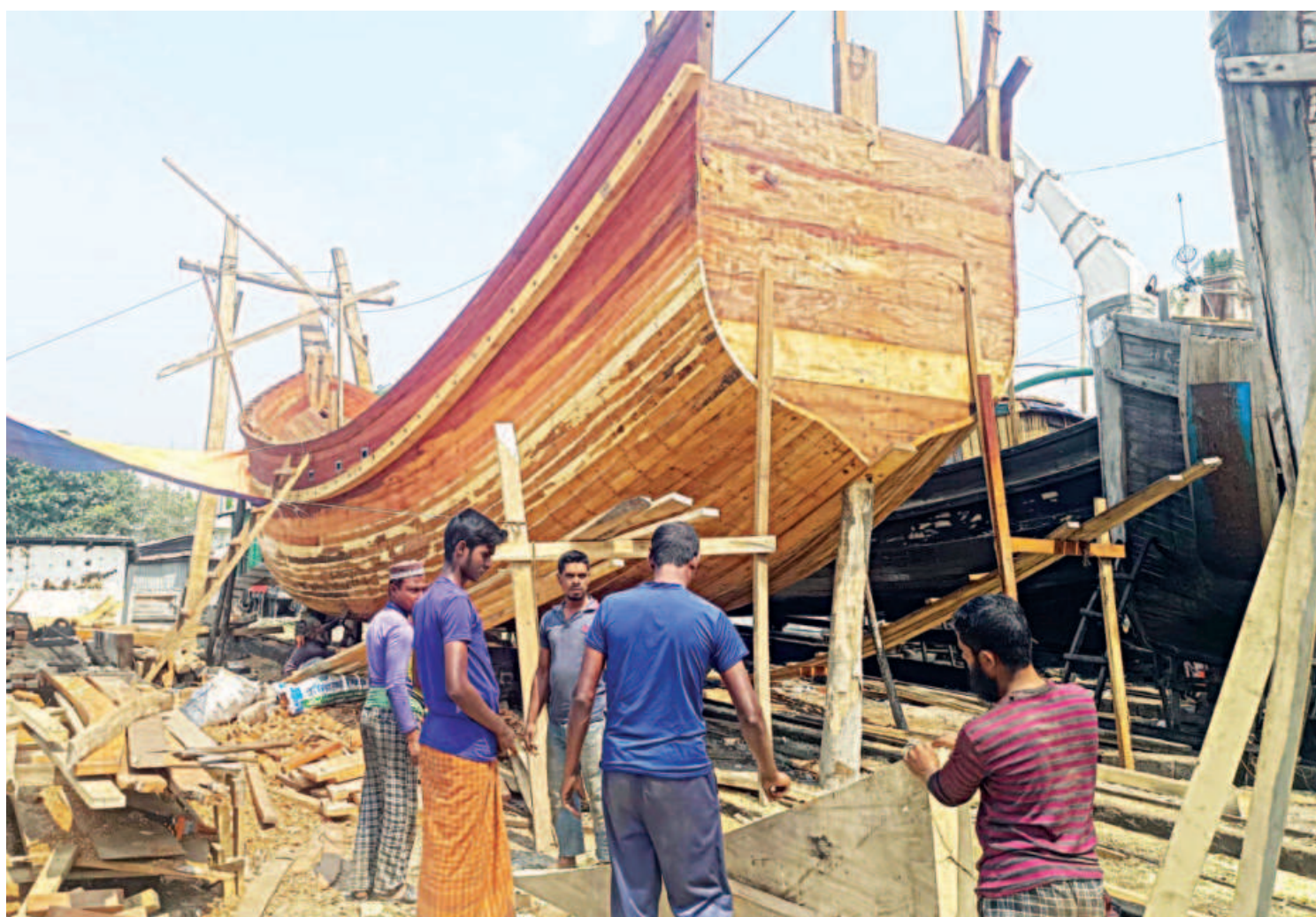
Labourers at a boatyard in Nizampur village under Kalapara upazila are seen working on the only wooden trawler being constructed so far this year. Ranging from 40 to 55 feet in length, each of these vessels can be used for sea fishing for about 10 years. PHOTO: SOHRAB HOSSAIN
