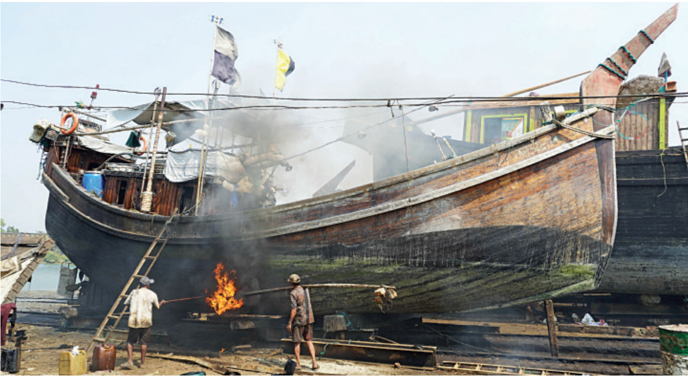
People conditioning the hull of a trawler with bitumen and fire in Majerghat area along the Bakkhali river in Cox's Bazar town. Any vessel that stays in the sea for a long time gets infested with barnacles that cause drag and reduce the vessels efficiency. The photo was taken recently.
