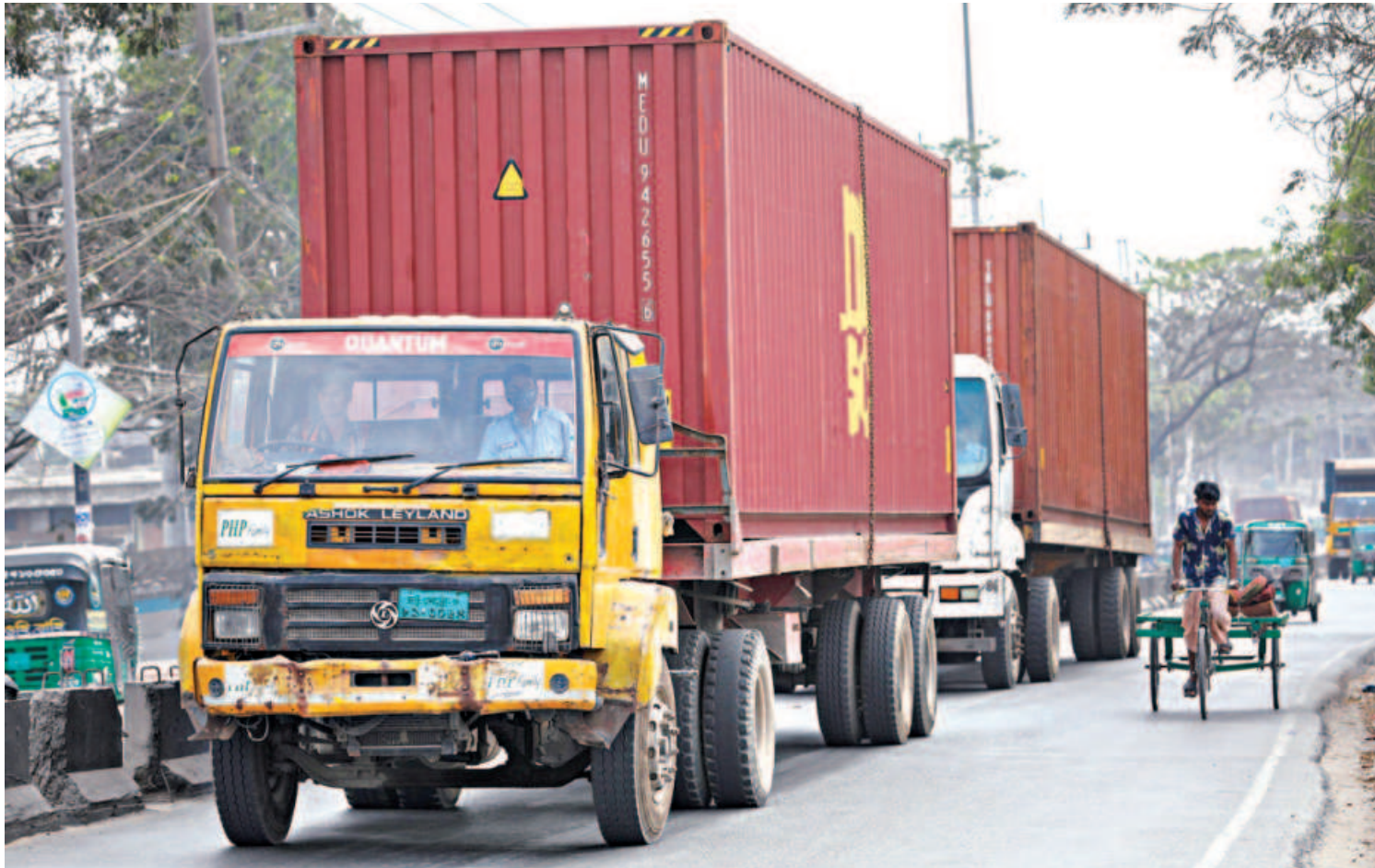
Prime movers, which are the front part of semi-trailer type trucks, can have engine capacities of around 5,660cc and pull loads of some 40 tonnes to 45 tonnes, including heavy machinery, import and export containers and goods meant for mega projects. According to market insiders, there are 7,850 prime movers in the country.
