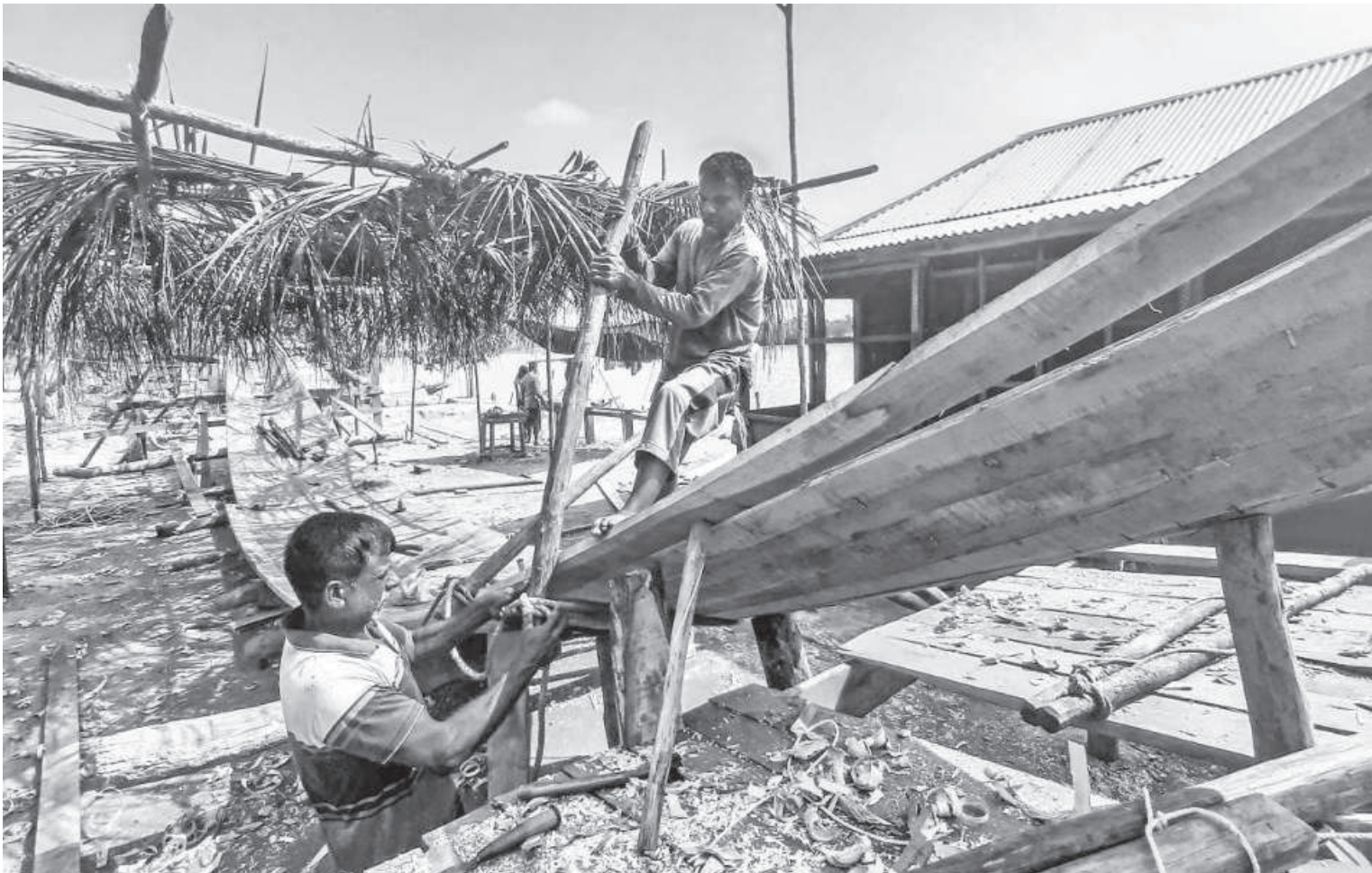
Hard at work, boat-makers are building the base of a fishing boat at Jelepara in Khulna's Dumuria upazila. After a month's work, the pieces of wood will become a 60-foot long and 12-foot wide vessel. Each one of these boats is traditionally made out of mahogany at a cost of Tk 6 lakh. This photo was taken recently.
